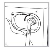
2. Connect the other end of the water inlet hose to the washer-dryer, screwing it onto the appliance's cold water inlet, situated on the top righthand side on the rear of the appliance (see figure).
